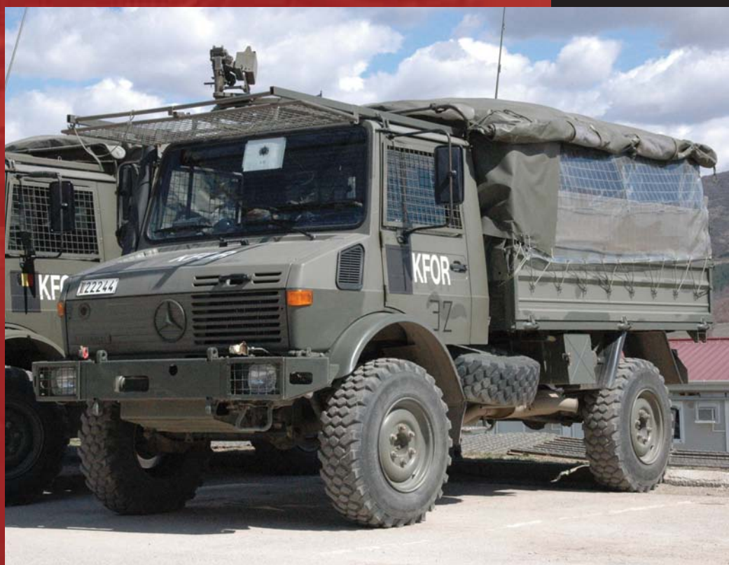
Below: Belgian Army U1550L in Kosovo fitted with basic anti-riot protection.
