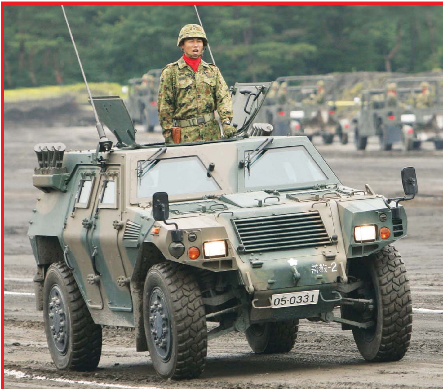
Above: a Company Commander's Vehicle, as distinguished by a larger antenna mounted above the driver's door and 76mm smoke grenade launchers. It is participating in a parade.
