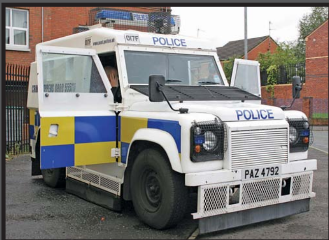
Below: the curved roof and flameproof bonnet design of PAZ 4792 identify it as a Ranger (Thetis) Mk.IV prototype.
