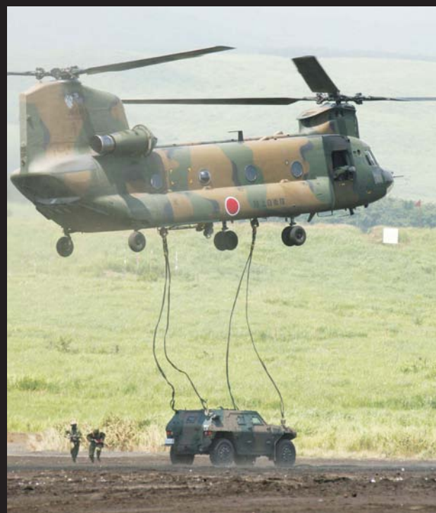
Above: the LAV is carried by the CH-47 Chinook as an under-slung load as it is too large to fit inside the helicopter internally.
