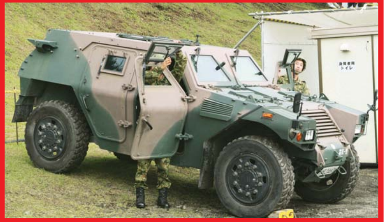
Above: observe how the faded brown paint has taken on an almost purplish hue on this LAV. This photo shows clearly how the door windows hinge open. Note that non-opening bulletproof side and rear windows are being retrofitted to standard LAVs.
