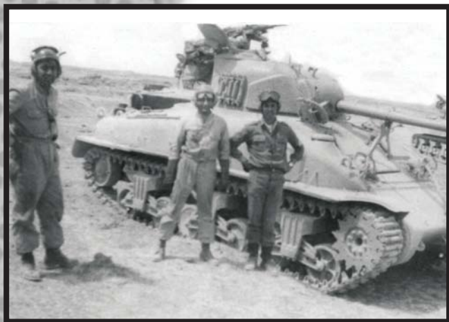
Above: the crew of a Chilean Army Sherman are pictured here taking a break during an exercise in the Atacama desert. Note the additional 'cheek' armour on the turret.
