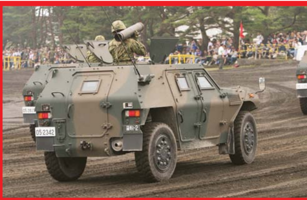
Above: the soldier is wielding a Type 01 Light Anti-Tank Missile (LMAT). The roof hatch consists of two semi-circular parts that open to either side.
