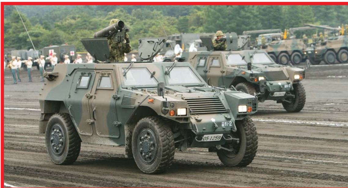
Above: a Company Commander's Vehicle, as distinguished by a larger antenna mounted above the driver's door and 76mm smoke grenade launchers. It is participating in a parade.
