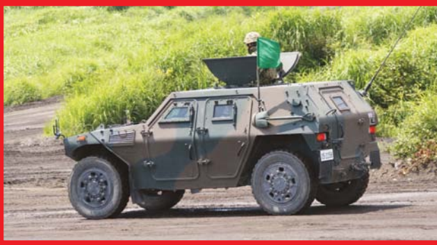
Above: an Anti-Tank Missile Vehicle rolls across the black volcanic soil that covers much of Japan. The green flag denotes it has already finished firing its live ammunition. A towing pintle is on the hull rear.
