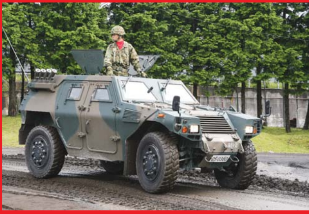
Above: the primary difference between the Company and Platoon Commander's Vehicles is the antennas. The latter does not have a large antenna fitted above the door, but instead an antenna is fitted at the rear.
